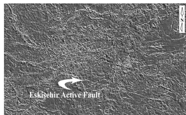
Figure 3. The active fault of the region on the PC2 transformed image with 4 major directions
