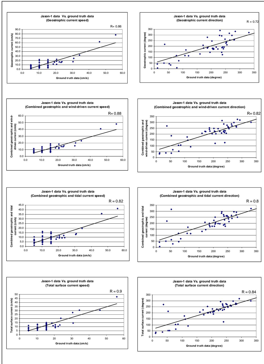
Figure 1: Regression lines between the derived surface current speed and direction with ground truth data.
