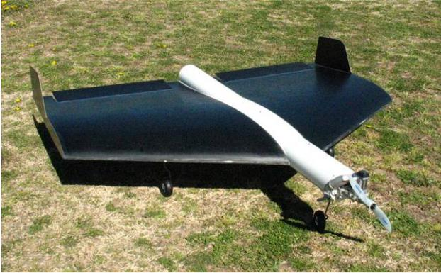
Figure 2. ITHACA UAV - Carbon fiber, ICE engine version (2008)
