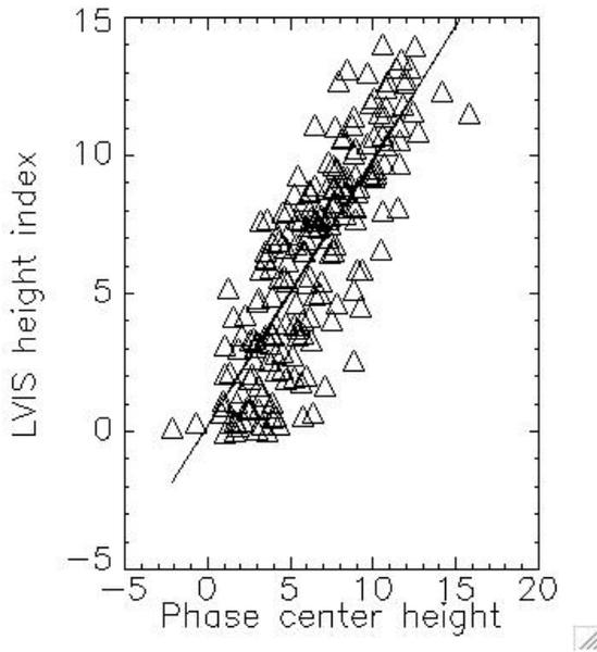
Figure 6. The correlation between 50% energy height (H50) and the phase centre height.
