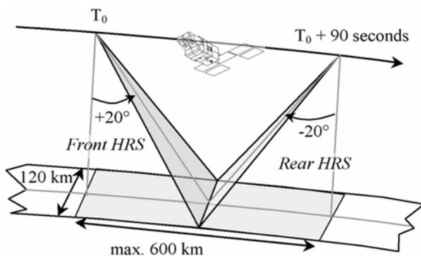
Figure 1. SPOT 5 HRS sensors acquisition process
