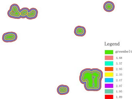
Figure 4 Temperature decrease value of greenbelt system on surrounding environment on June 12, 2004
