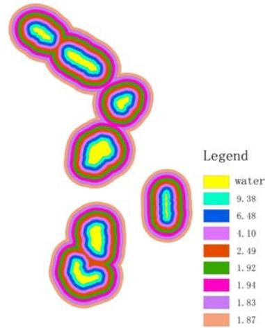
Figure 6 Temperature decrease value of water system on surrounding environment on June 12, 2004
