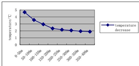
Figure 5 Statistic map of temperature decrease of greenbelt impacting on surrounding environment
