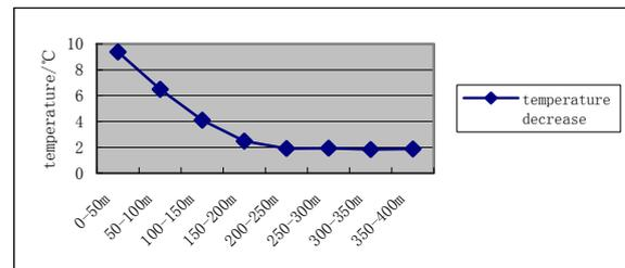
Figure 7 Statistic map of temperature decrease of water impacting on surrounding environment
