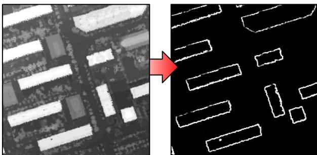
Figure 5: some areas already cover by LiDAR data and by applying texture analysis clear buildings boundaries will show.
