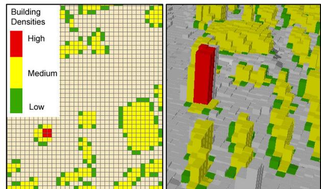
Figure 10: 3D simulation presents the Union between BCR and FAR ratios.
