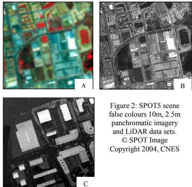
Figure 2: SPOT5 scene false colours 10m, 2.5m panchromatic imagery and LiDAR data sets.
