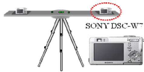
Figure 7. Close range photogrammetric system using amateur digital camera
