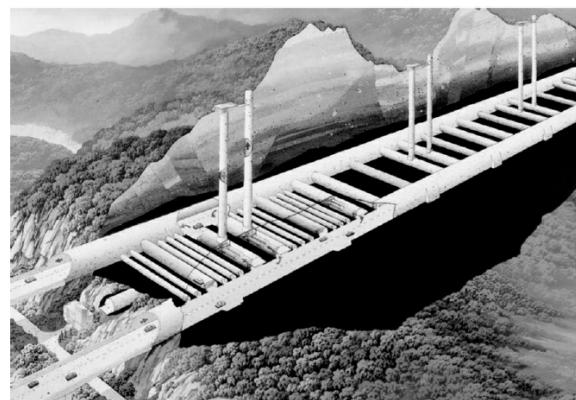
Figure 2. Ventilation System of Hsueh-Shan Tunnel
