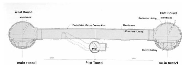
Figure 3. Relationships of Hsuehshan Tunnel and Pilot Tunnel
