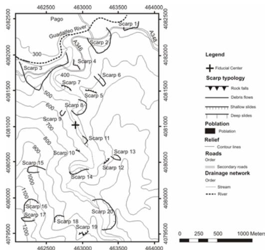
Figure 2. Landslide crowns of zone (photogram) P5-5.
