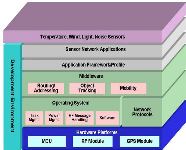
Figure 2. The architecture of hazard detecting WSN
