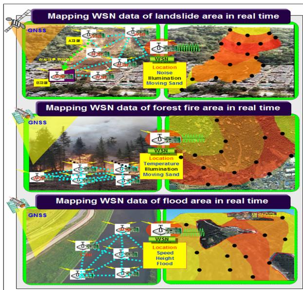
Figure 4. Mapping hazard data from WSN
