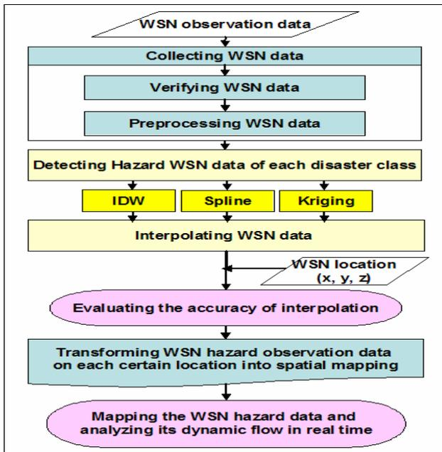
Figure 3. Transforming WSN data into spatial data type
