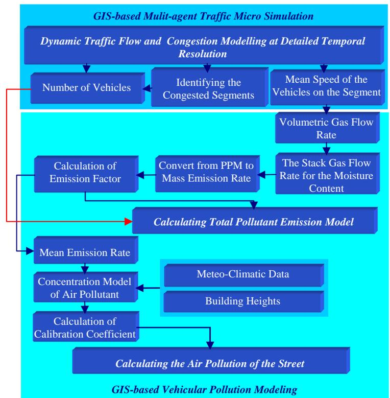
Figure 1. The proposed work flow of the GIS-based multi-agent traffic micro simulation for modelling the street air pollution
