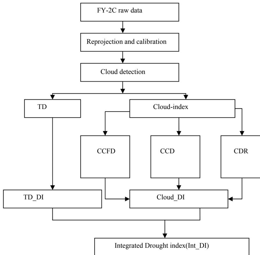
Figure 1. The flow chart of the model
