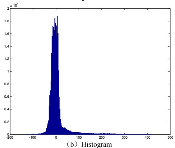
Figure 4. Height difference of InSAR-DEM and GPS-DEM
