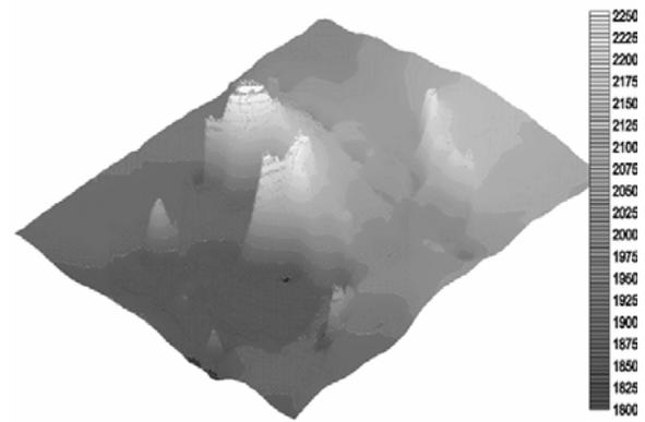
Figure 3. DEM from the topographic points obtained during the field survey
