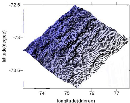
Figure 6. Contour map without tilt correction (interval: 20m)
