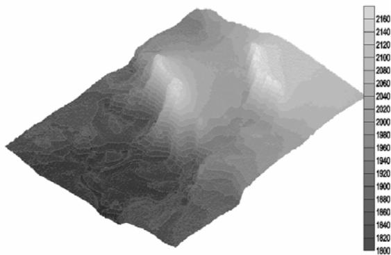
Figure 2. DEM generated using tandem SAR image data
