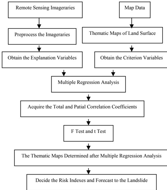
Figure.2 Technical flowchart of monitoring landslide disaster using remote sensing
