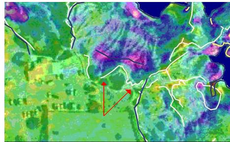
Figure 3. Chromostereographic representation of changes (in this case material loss), superimposed to the stereoplotted lines of different time periods and orthophoto.
