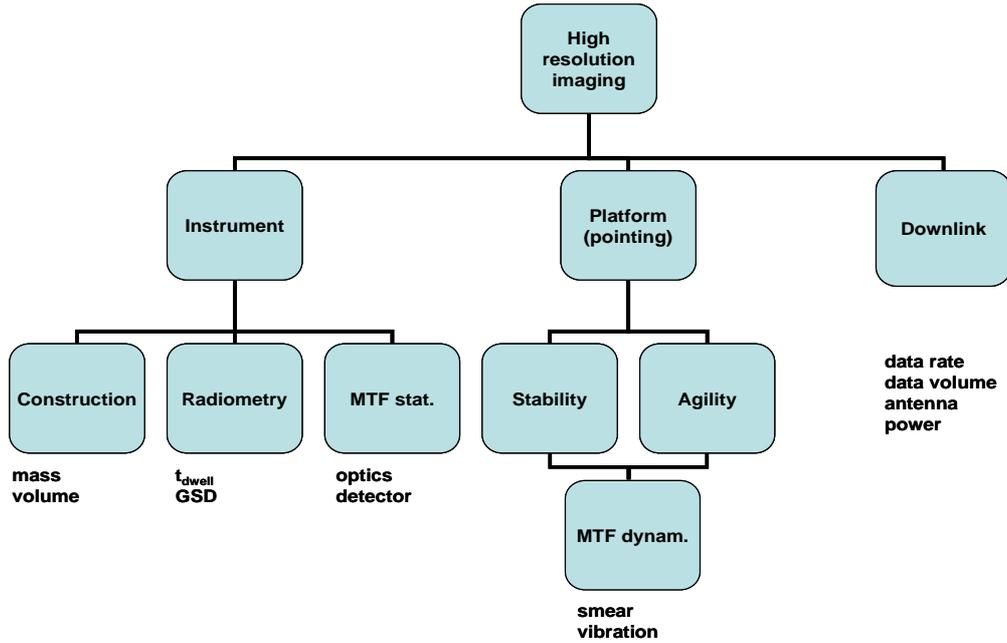
Figure 2. Components of a space borne mapping system and their influences on the system performance
