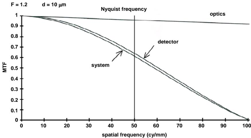
Figure 5 System MTF composed of  $MTF_{Optics}$  and  $MTF_D$
