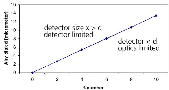
Figure 3. Airy disk parameter  $d$  as a function of the f-number  $F$  ( $\lambda=0.55 \mu m$ )
