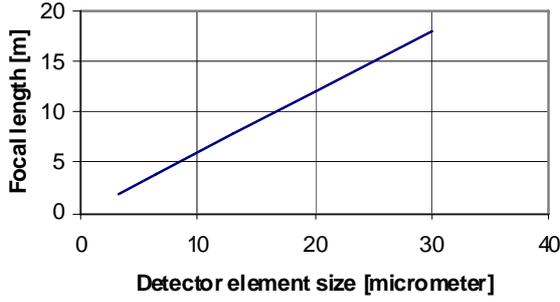
Figure 4. Dependence between detector element size  $x$  and necessary focal length  $f$  for a given ground pixel size of  $X = 1$  m from an orbit altitude of 600 km  $MTF_D$  of the detector element with size  $d$  is described by the sinc function (in  $x$ -direction)
