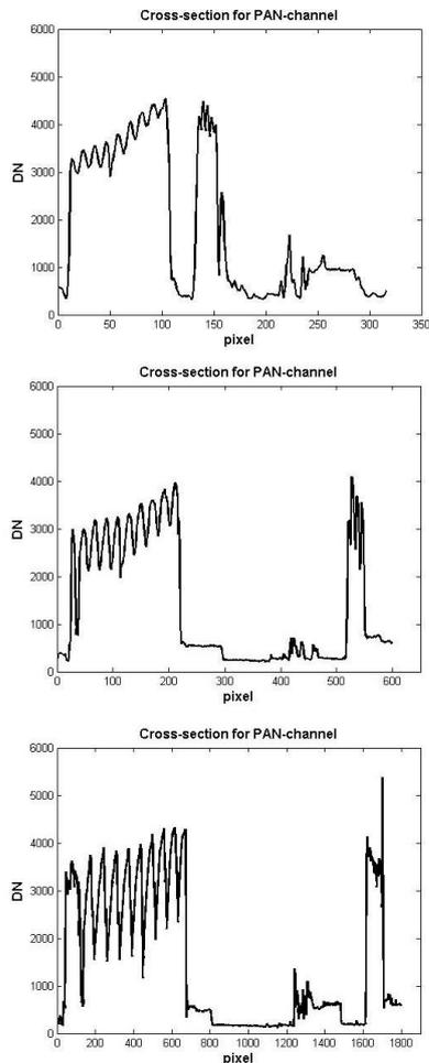
Figure 8 - Radiometric response of the panchromatic channel from three images from the same object area and different GSD
