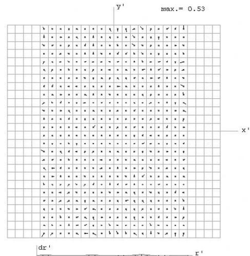
Figure 9 - Remaining image residuals less than  $0.53 \mu\text{m}$  after the least squares adjustment including additional self calibration parameters
