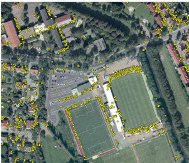
Figure 7. TerraSAR-X persistent scatterer for urban area without deformation
