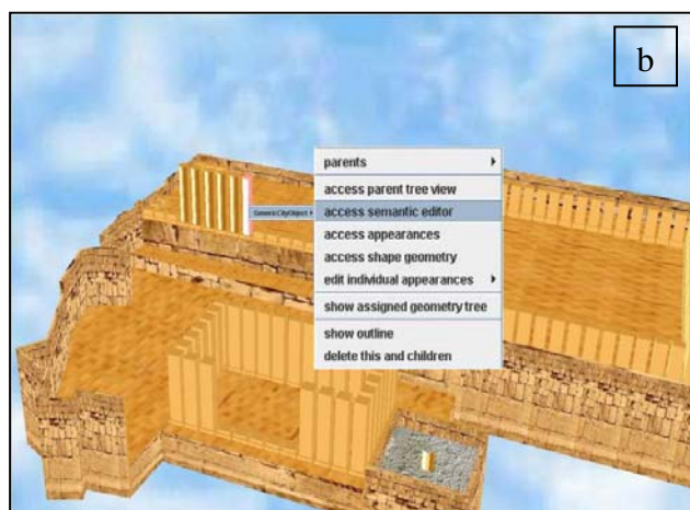
Figure (6.b): The possibility to add thematic information using a semantic editor (screen)
