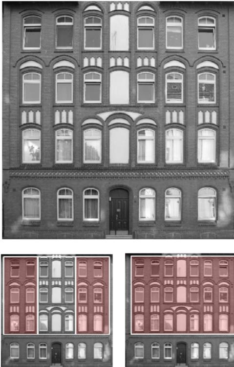
Figure 5: Two structural decompositions of a façade
