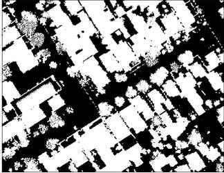
Figure 6. Binary image representing the aboveground objects.
