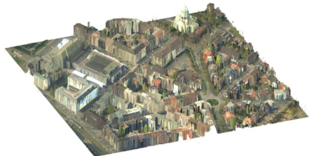
Figure 3: A 3D view of dataset; height of objects are obtained using the first pulse laser range data
