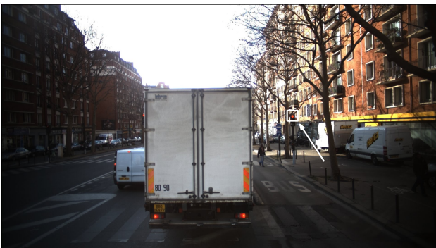
Figure 9: A false detection example. Red light of tri color light is detected as wrong way traffic sign.
