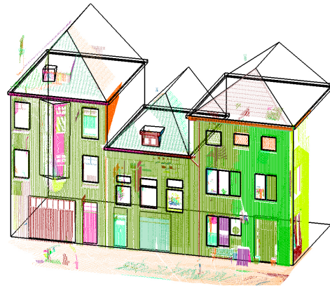
Figure 2: A reconstructed building facade model, shown together with segmented laser points
