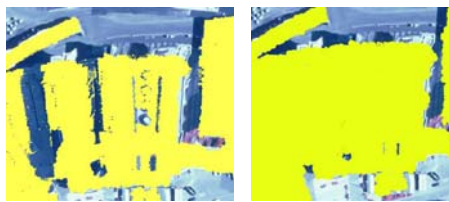
Figure 7. Left: buildings without the regions which covered by shadow in ((1 \cap 2) \cap 4) , Right: more complete roofs with ((1 \cap 2) \cap 4) \cup 3 .
