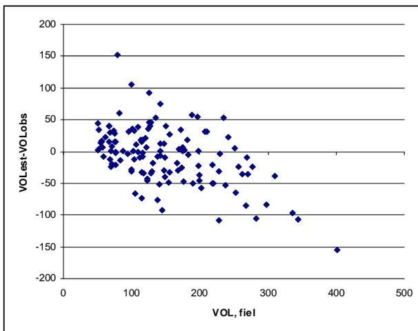
Figure 2. Volume estimation errors ( $Vol_{Est}-Vol_{Obs}$ ) with best performing ALS data set.
