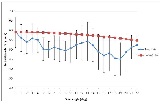
Figure 5. ALS results for asphalt road in the Espoonlahti harbour. The blue line is the raw data at 500m altitude, each point is an average of several points having the same incidence angle. The error bars represent the standard deviations of the average.
