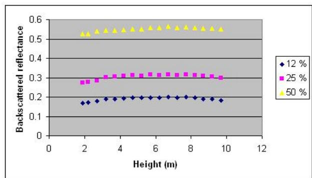
Figure 7. Backscattered reflectances measured with the FARO LS in a scissor lift at different heights. The results are presented for Spectralon targets of 12%, 25%, and 50% reflectance.
