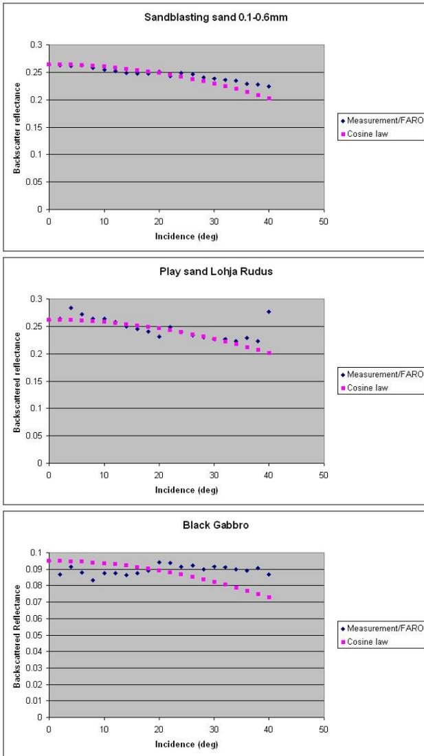
Figure 4. TLS results for sand and gravel targets: sandblasting sand with 0.1-0.6mm grain size (top), play sand (Lohja Rudus Ltd.) (middle), and black gabbro gravel (bottom).
