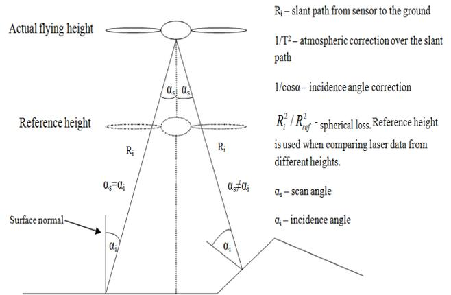
Figure 1. The incidence angle and the scan angle. Some of the ALS intensity atmospheric correction parameters are also shown (cf. Eq. 1).
