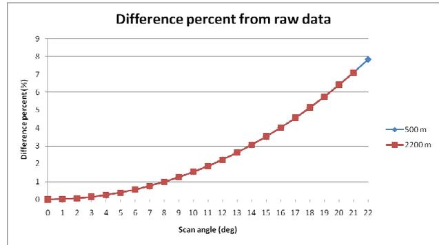
Figure 6. Effect of the cosine correction on intensity values (difference between raw and cosine corrected data).
