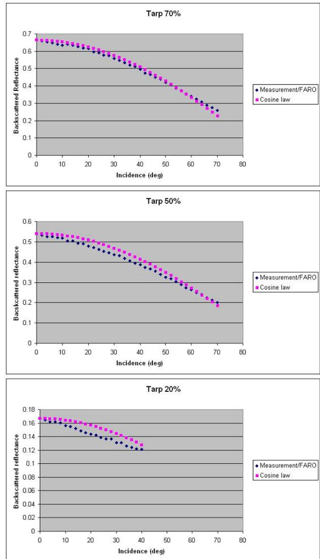
Figure 3. TLS results for brightness tarps of 70% (top), 50% (middle), and 20% (bottom) nominal reflectance.
