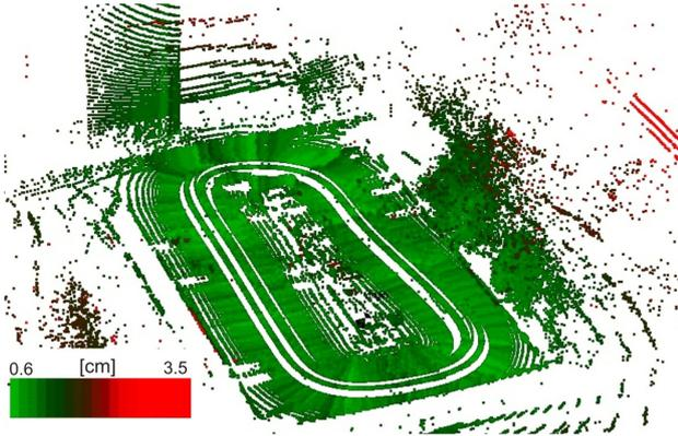
Figure 3: Stochastic point cloud with points colored related to the mean coordinate uncertainty  $\bar{\sigma}$  (Eq. 27)
