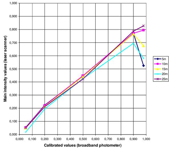
Figure 7. Relation between calibrated values (photometer) and recorded intensity values by HDS 6000
