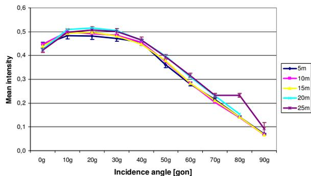
Figure 9. Mean intensity in dependence on incidence angle (reflectivity 50%)
