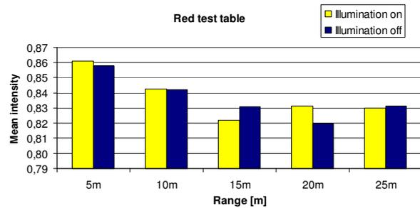
Figure 11. Mean intensity values (red test table) in dependence on distance and ambient lighting conditions
