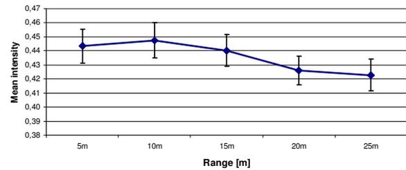
Figure 8. Mean intensity  $I$  and its standard deviation  $\sigma_I$  in dependence on the distance (reflectivity 50%)
