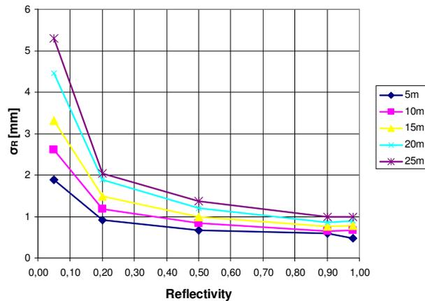
Figure 4. Standard deviation  $\sigma_R$  [mm] of range measurements in dependence on reflectivity
