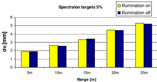
Figure 6. Range accuracy  $\sigma_R$  in dependence on ambient lighting conditions (reflectivity 5%)
