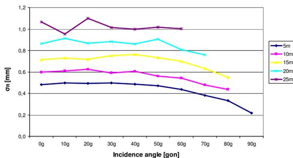
Figure 10. Standard deviation  $\sigma_R$  [mm] of range measurements in dependence on incidence angle (colour red)
