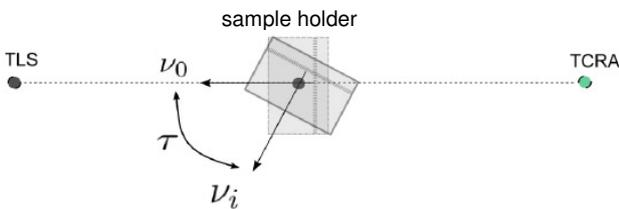
Figure 2. Top view of the test configuration. Rotation of the sample holder in defined angles  $\tau$  to realize different incidence angles (related to the  $0^\circ$ -direction  $\nu_0$ )
