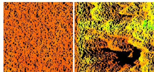
Figure 13. Oblique view on the point cloud acquired from a aluminium plate (left part) and a copper plate (right part)
