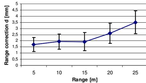
Figure 3. Range correction value  $d$  and its uncertainty in dependence on distance (target of 50% reflectivity)
