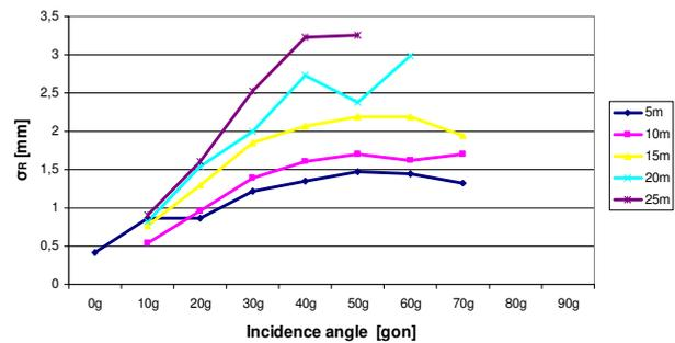
Figure 12. Standard deviation  $\sigma_R$  of range measurements for aluminium in dependence on incidence angle
