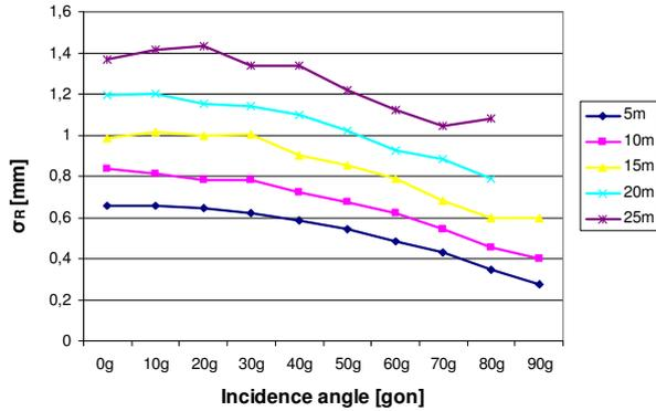
Figure 5. Standard deviation  $\sigma_R$  [mm] of range measurements in dependence on incidence angle (reflectivity 50%)
