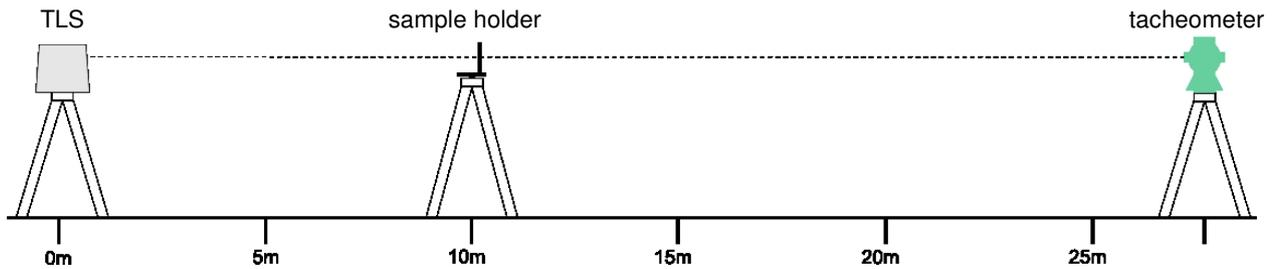
Figure 1. Test configuration TLS, sample holder and tacheometer (reference measurements)
