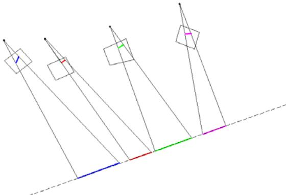
Figure 4. A case where intersecting plans do not correspond to a single 3D line segment
