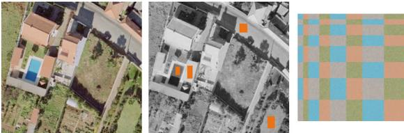
Figure 2. Signature image (left) with 4 land cover types (centre) and the resulting synthetic image (right).
