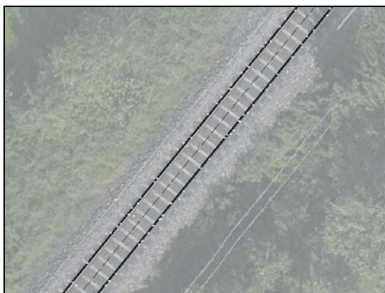
Figure 6. Ortho-image overlaid with the extracted rail tracks: rail (solid), rail centre line (dashed) and filtered rail points (white) (right)
