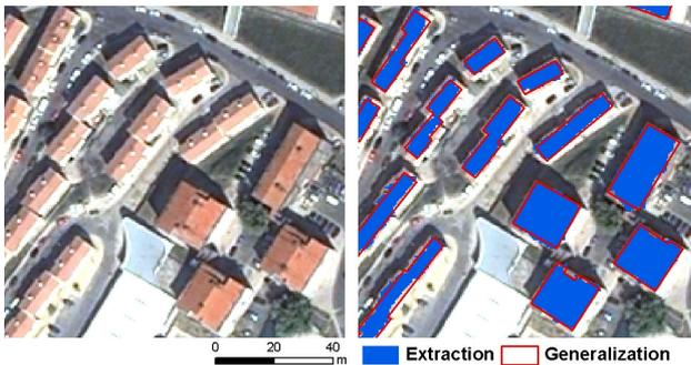
Figure 4. Detail of red tile roofs in study area and their extraction and generalization
