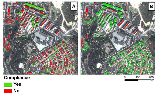
Figure 5. Compliance map for planimetric tolerance for scales 1:5 000 (A) and 1:10 000 (B)
