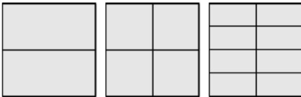
Figure 1. Division into tiles for two, four and eight threads
