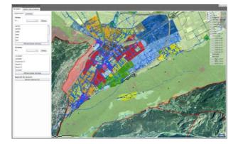
The client who uses SyGEMe can watch the attributes of the network objects. On the web platform, different layers include geographical objects whose details can be consulted. We can mention here data of the pipes (diameter, construction year...), valves, tanks (size...) zones attributes and many others. That information is centralized in a database and available in any time.
