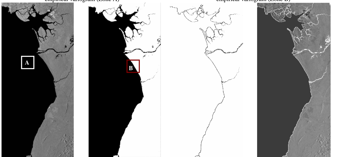
(a) Original image (b) Extraction of the class Sea (Black color) (c) Extraction of the coastline (Black color) (d) Result of the fusion applied after extraction of the coastline
