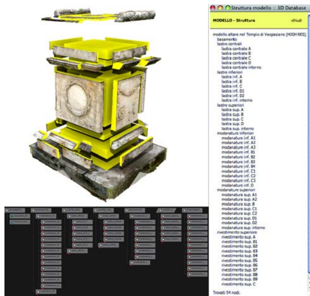
Figure 5. Semantic fragmentation of a 3D model of a find and organization and naming of its sub-elements. Each sub-element corresponds to a single node and its linked file within the database. On the right, the node organization within the information system interface. Each row is a hyperlink that connects the sub-elements to its data sheets; on the left, the fragmentation of the 3D model and the organization of the sub-elements in groups within the modeling interface.
