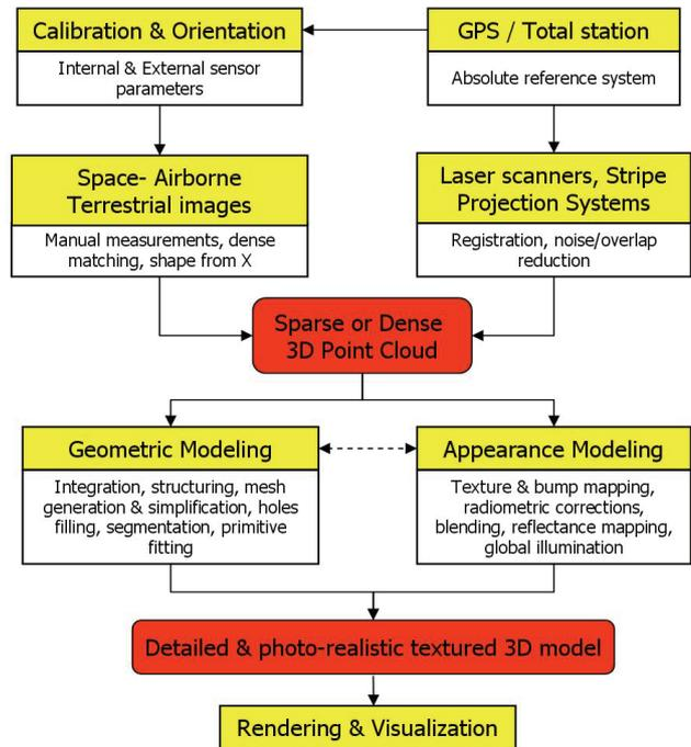
Figure 2: 3D modelling pipeline for site documentation.
