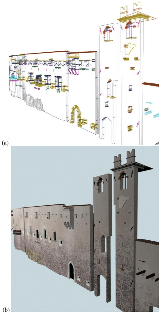
Figure 5: Architectural elements extruded from rectified images with CAAD tools (a); the final texture model of the façade (b).
