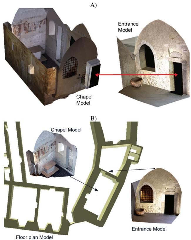
Figure 8: Model registration with common portal (A) or using floor plans (B).
