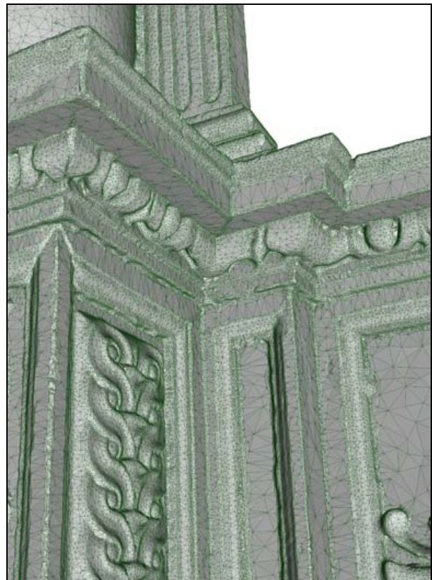
Figure 7 – 8. Top: the file with a tolerance of 0.02 mm. Bottom: the file "lightened", with tolerance of 0.2 mm.
