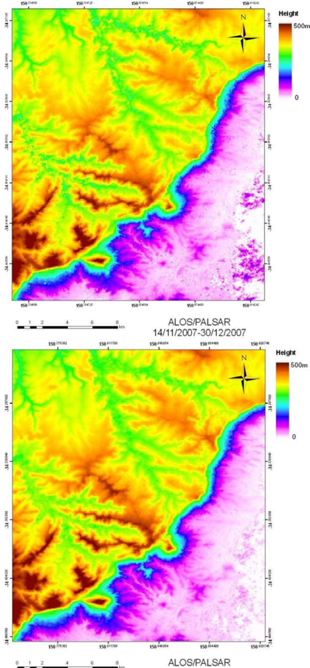
Figure 3. InSAR DEM generation using ALOS PALSAR data: (upper) single pair acquired on 14/11/2007 and 30/12/2007; and (lower) an average DEM of 5 interferometric pairs for Wollongong, NSW.
