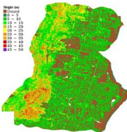
Figure 2. Canopy Height Model (CHM) showing the maximum height of the tree canopy in metres, generated by subtracting the DTM from the DEM.
