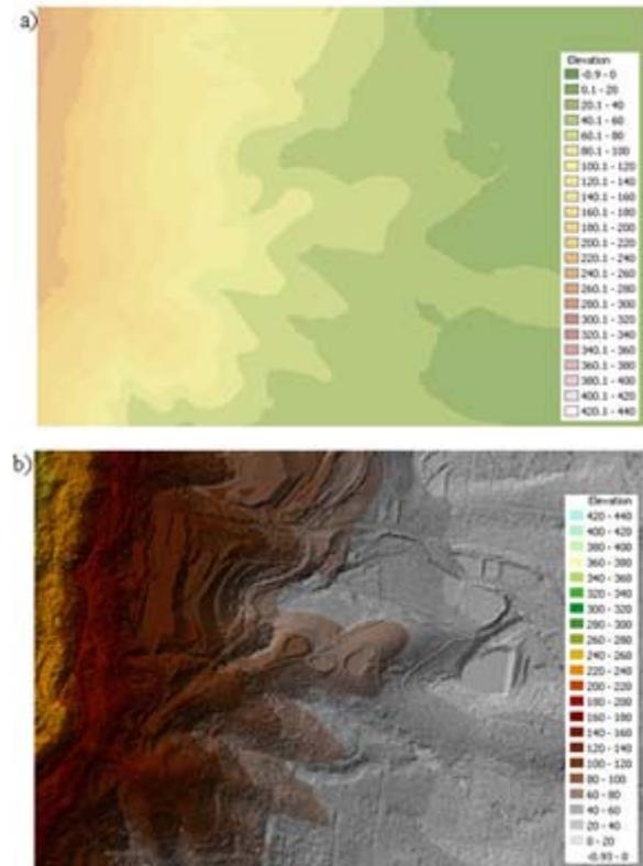
Figure 1. Comparison of approaches to interpolation of height surfaces using LiDAR data: a) Grid based Natural Neighbour (NN) interpolation; and b) Triangular Irregular Network (TIN).
