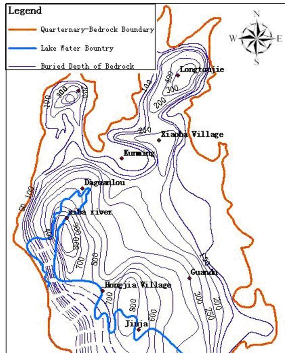
Figure 3. The buried depth of bedrock of Kunming Basin
