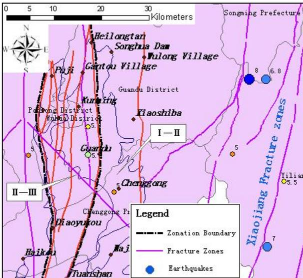
Figure 2. Main fracture zones and crust activity zonation of Kunming Basin
