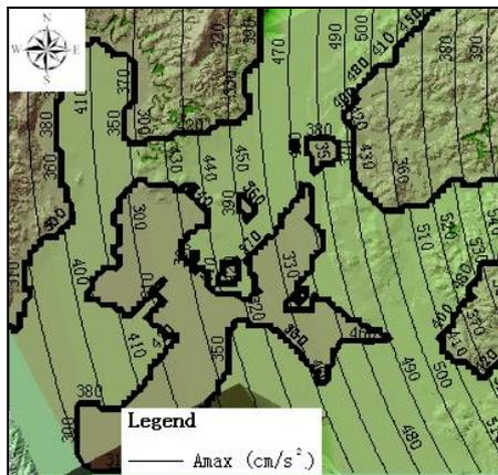
Figure 5. The peak horizontal acceleration corresponding to the seldom happen earthquake.
