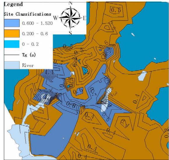
Fig.4 The characteristic period  $T_g$  and site classifications of Kunming Basin.
