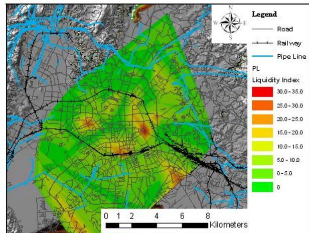
Figure 7. The ground liquefaction risk of Kunming basin in seldom happen earthquake (Japan Model)
