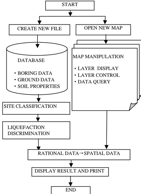
Figure 6. Flow chart of the GIS-based liquefaction prediction system developed in this paper.
