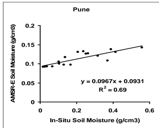
Figure 4. Correlation of in Situ Soil Moisture and AMSR-E Soil Moisture
