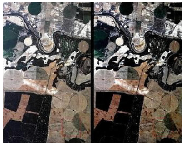
Figure 4: Original DN image (left) and atmospherically corrected reflectance (right).
