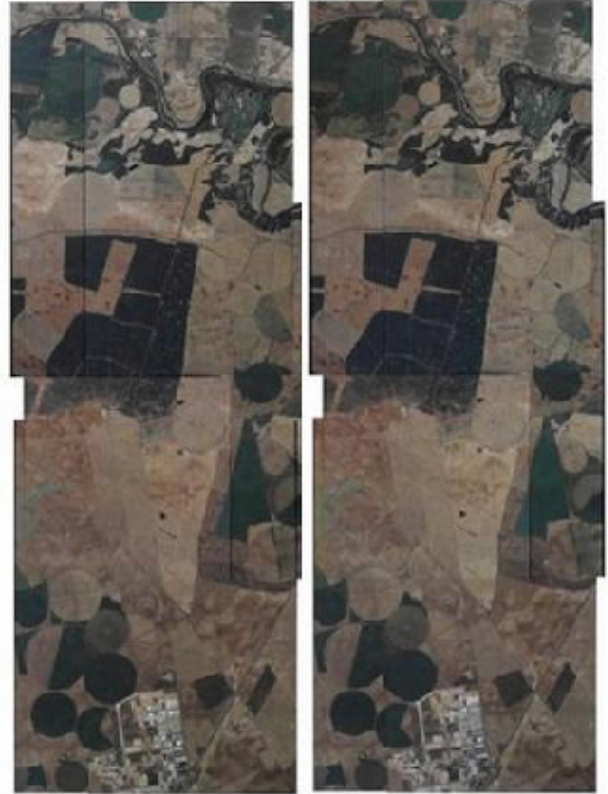
Figure 3: Original Orthoimage (left) and homogenized (right) applying the Lidense geometric kernel.
