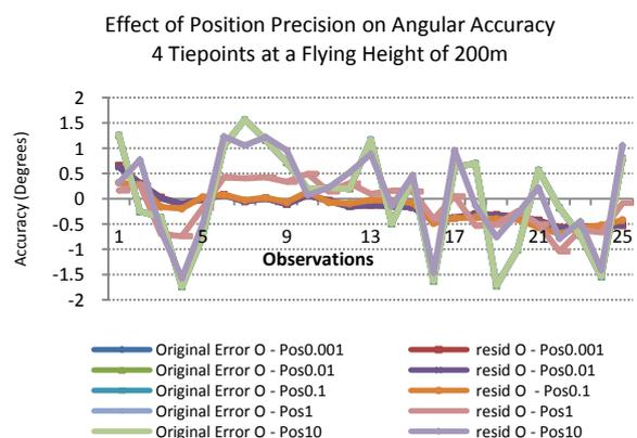
Fig. (3): Orientation accuracy at different position precision – Forward Kalman Filtering
