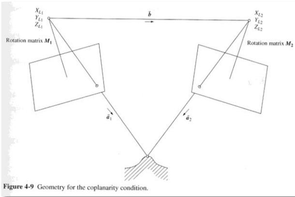
The co-planarity condition is based on the fact that the volume ( $V$ ) of the parallelepiped (a polyhedron consisting of all parallelogram faces) of three co-planar vectors will be 0 as shown in equation 2 below.
