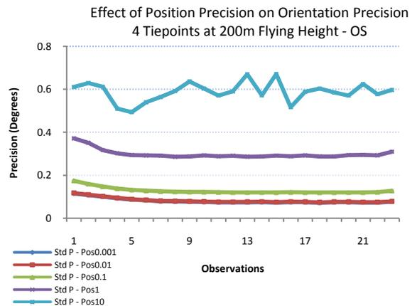
Fig. (2): Improved orientation precision due to improved position precision – Backward Optimal Smoothing
