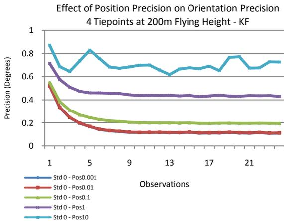
Fig. (1): Improved orientation precision due to improved position precision – Forward Kalman Filtering
