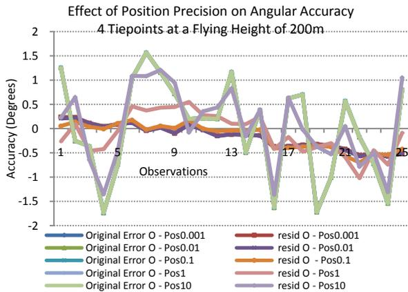
Fig. (4): Orientation accuracy at different position precision – Backward Optimal Smoothing
