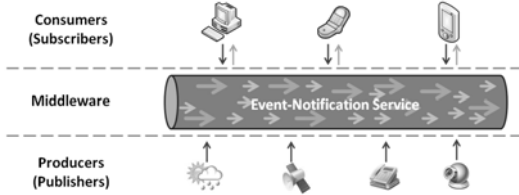
Figure 1: Publish/Subscribe system components
