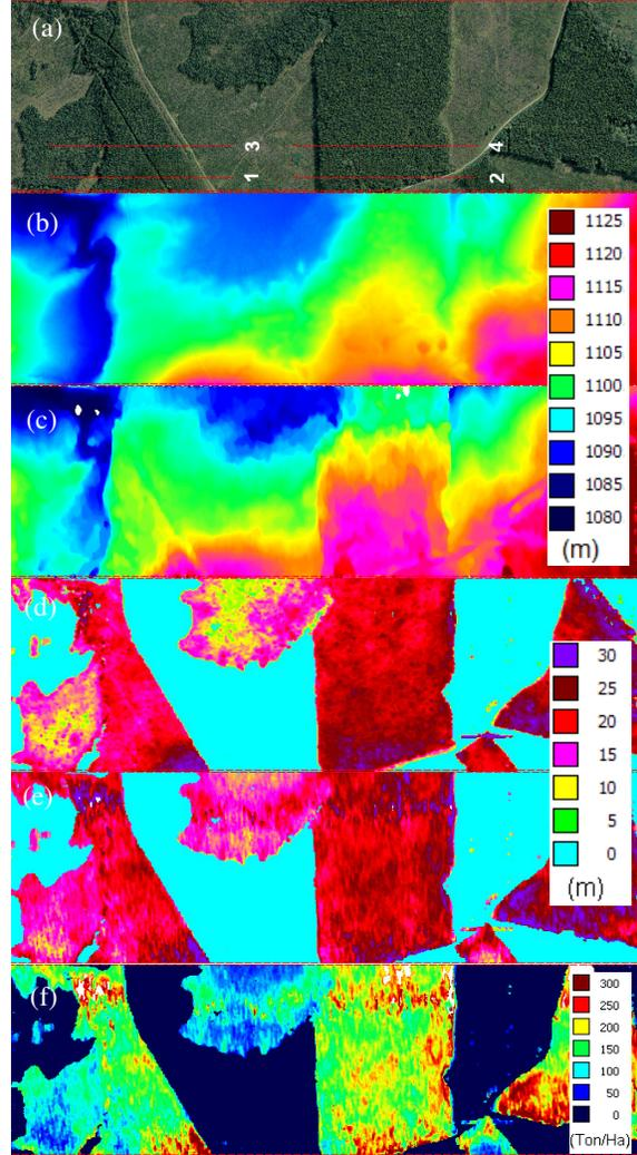
Figure 2. (a) Profiles on the air photo, (b) Lidar bare-earth DTM, (c) L-Band DTM, (d) Lidar tree height map, (e) L-Band estimated tree height map (f) Biomass estimated from (e)
