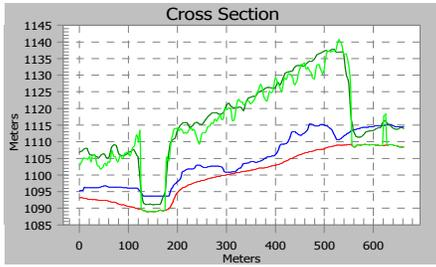
Figure 3. Elevation profile of Line 1 in Fig. 2(a): red – Lidar DTM, dark green – Lidar  $h_{100}$ , light green – L-Band tree height, blue – L-Band ground. Note that the tree height profiles are with reference to the underlying DTM.
