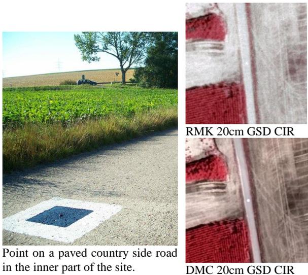
Figure 2: Signalized point within RMK and DMC images.
