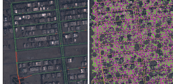
Figure 7. Left: the results of evaluation Green: evaluated roads. Red: rejected roads. Right: Seeds and all possible connections.
