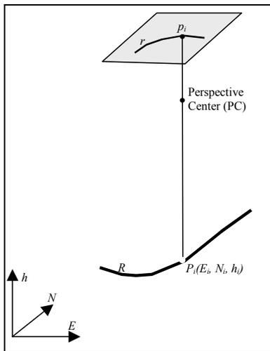
Figure 1. Object-space road model principle for a single aerial image
