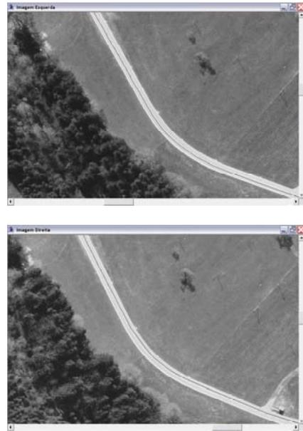
Figure 3. Extraction of a road segment from a stereo sub-images.
