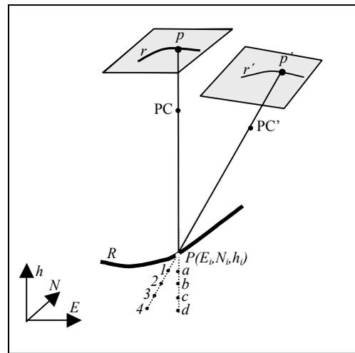
Figure 2. Object-space road model principle for a stereo pair of aerial images.
